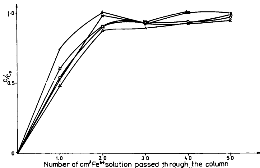
Fig. 7. Iron exchange performance of samples prepared by irradiation under vacuum. Variation in C/C_0 (see text) with variation in the volume of Fe(III) solution passed through a column. (●) [-COOH] , 2.2 \text{ meq g}^{-1} ; (○) 2.61 \text{ meq g}^{-1} ; (□) 2.89 \text{ meq g}^{-1} ; (×) 3.28 \text{ meq g}^{-1} ; (Δ) 3.66 \text{ meq g}^{-1} .
